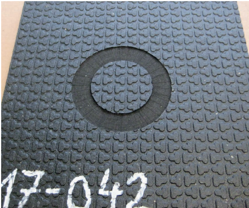
Figure 5: Test sample after abrasion test
